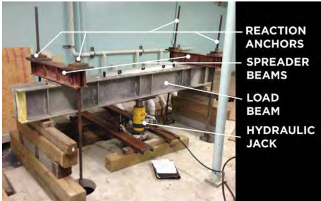
INDOOR COMPRESSION TEST FIGURE B-4
